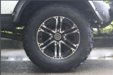
12 inch aluminium alloy rim with all terrain tire (For Lifted Golf Cart)
