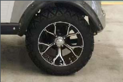
14 inch aluminium alloy rim, all terrain tire: Tire dimension: 22*10-14 (For Lifted Golf Cart)
