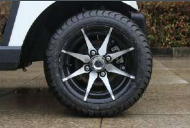
12 inch aluminium rim wheel with low profile tire 215/35-12 (Optional for 2-4 seats, standard for 4 seats with cargo box and 6 seats)
